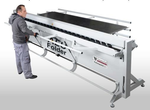
• The locking and folding feet are completely adjustable and are made of plastic that will not mark or scratch the surface of the composite panel during the bending process, even when folding of all four sides.
